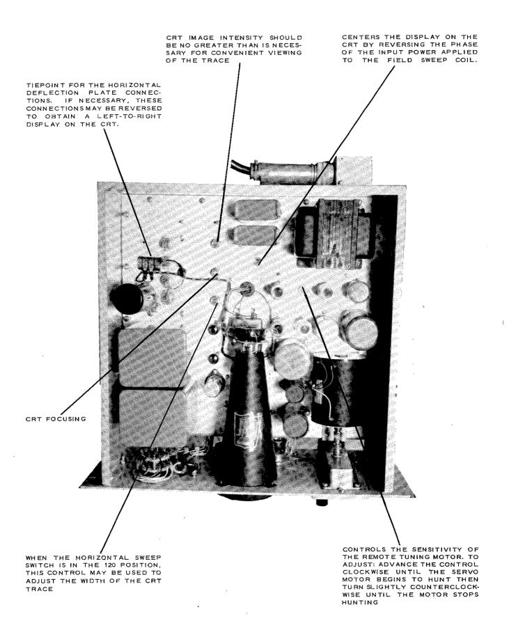
FIGURE 4. DISPLAY AND CONTROL UNIT ADJUSTMENTS
