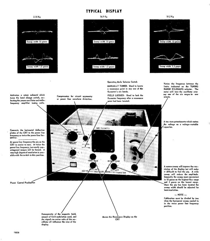
FIGURE 1. THE DISPLAY AND CONTROL UNIT
